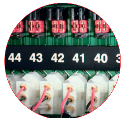
Detail view of normalling pod settings. All units supplied half-normalled and bussed grounds as viewed above.
